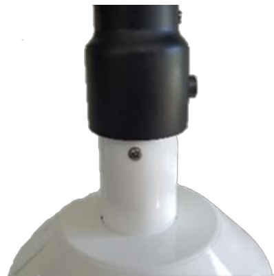
Figure 14: Miniaervane properly installed
