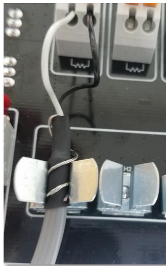
Figure 18: BOM cable inserted into 360° shield connection
