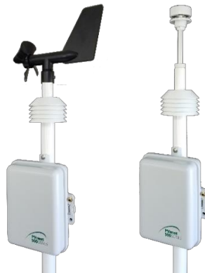
Figure 4: PVmet-500Series with a Miniaervane and ultrasonic anemometers
