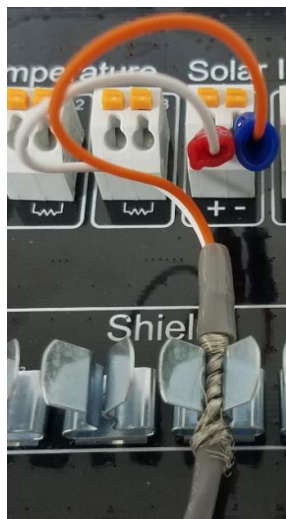
Figure 20: Solar irradiance sensor shield connection
