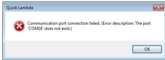
Error Message: Communication port connection failure
